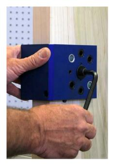
Use the supplied 3/8" socket cap screw to fasten both templates together. Just snug the two plates together.
