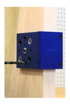
We will be drilling the most popular retrofit holes for this installation. Two 5/16" diameter holes located at 6:00 and 12:00. The procedures will be the same for the other holes. Drill the two holes half way from both sides of the door. When drilling, back the drill out several times to help remove chips. See the chart on the back page for other locks that can be installed with this drill guide.
