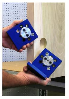
The template set consists of both inside and outside drill guides. All required holes are lined with hardened bushings.
