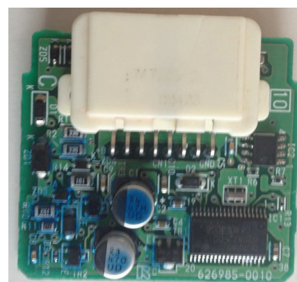
Immobilizer control module Tokai Rikka. It is with EEPROM 93C66. Dump is ENCRYPTED!
