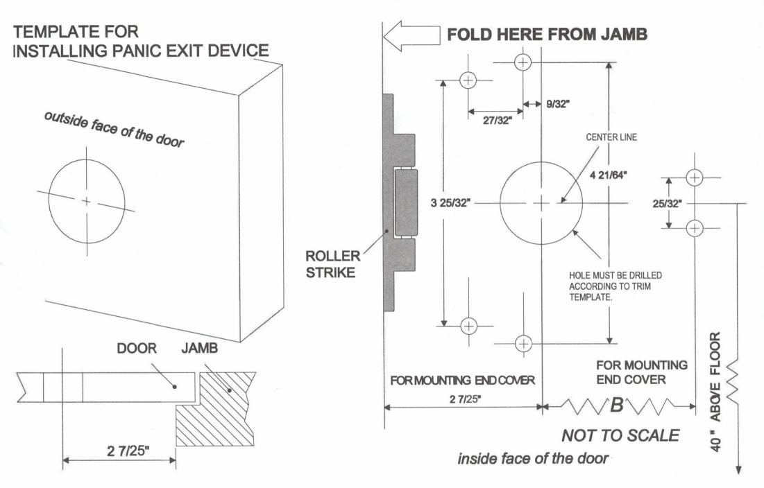
(A)For UL-500 Series (UL Listed)-Drill & tap for (6) 1/4"x20 machine screws for Exit Device and Drill & tap for (3) 1/4"x20 machine screws for Roller Strike.
