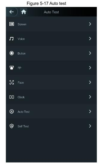
When you select Auto Test, the access controller will guide you to do all the auto tests.
