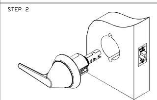
INSTALL INSIDE LOCK ASSEMBLY IN CUTOUT, LINE UP RETRACTOR ON LOCK BODY WITH LATCH (NOTE- EASIER TO DO THIS WITH THE LATCH LOOSE AND THEN SCREW IN THE LATCH AFTER THIS STEP)
