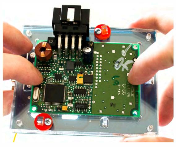
Push down the immo board on to the Click'n Go adapter. Make sure it's mounted correctly.
