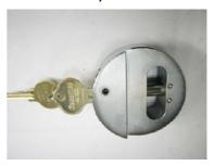
2. Pull out the whole cylinder and take an allen key.
