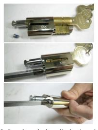
10. Put the whole cylinder into lock body.
