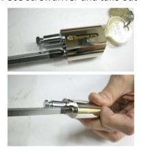
6. Pull out the cylinder from housing.
