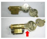
9. Put the cylinder into the housing.
