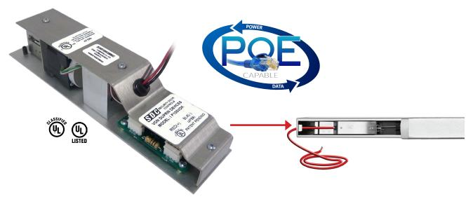
The SDC IP100 Series 12V PoE-Capable Electric Latch Retraction Kit enables electric access control and dogging of mechanical exit devices. When energized the motor retracts the exit device latch and pulls the pushpad\* into the dogged (depressed) position enabling momentary or sustained push and pull operation of the door.
