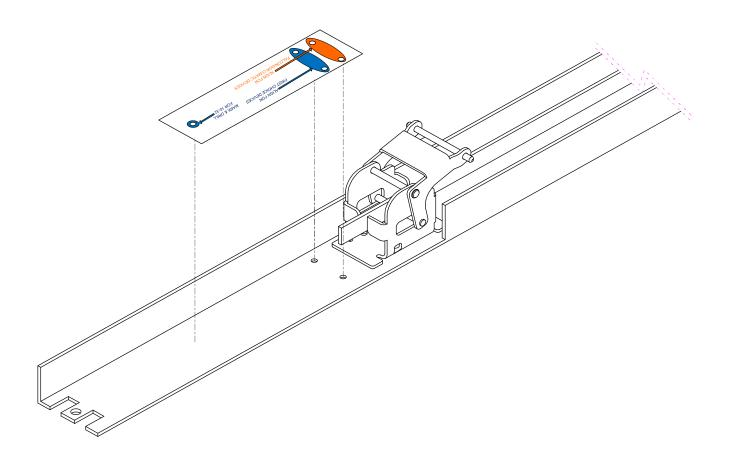
USE TEMPLATE WHEN DEVICES ARE LONGER THAN 36" FOR ADDED STABILITY OF KIT.
