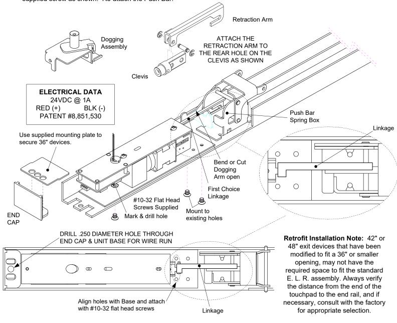
When retrofitting to existing vertical rod devices, adjustment of the rods is required for proper operation of the Electric Latch Retractor. Once the unit is properly installed, energize it so the push pad is dogged down, then reconnect the vertical rods to the device and make the proper adjustments.
