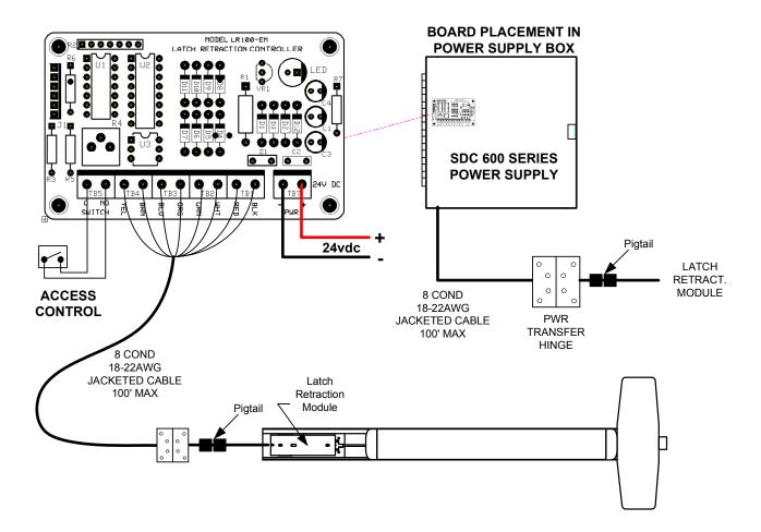
**Retrofit Installation Note:** 42" or 48" exit devices that have been modified to fit a 36" or smaller opening, may not have the required space to fit the standard E. L. R. assembly. Always verify the distance from the end of the touchpad to the end rail, and if necessary, consult with the factory for appropriate selection.
