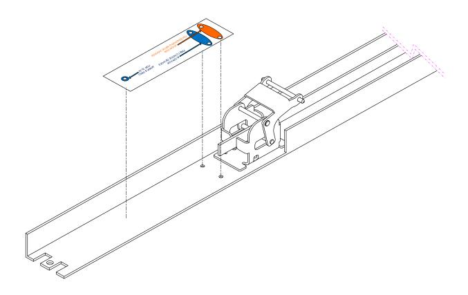
ALIGN TEMPLATE TO EXISTING HOLES, FALCON/DOR-O-MATIC or FIRST CHOICE MARK AND DRILL 1 HOLE FOR 10-32 FLT HD
