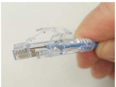
Then remove the terminated RJ45 plug from the crimping socket. Quickly inspect that all wires have been closely trimmed to the plug in the front.
