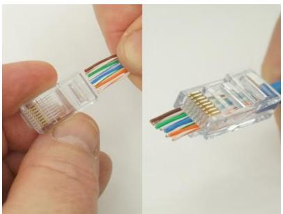
Hold the RJ45 plug upside down (strain relief clip facing down). Insert the wires into the back of the plug until they come out the front of the plug at least ½ inch (1.27cm).
