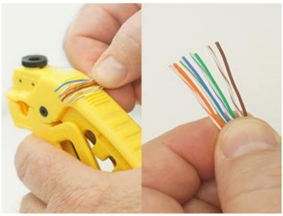
Straighten each wire conductor.
