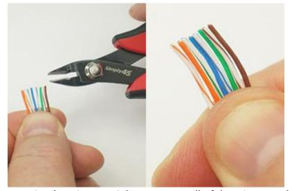
Using a flush cutter, trim the wires straight across so all of the wires are the same length.
