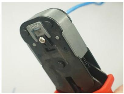
The Simply45 crimper is a ratcheted crimper. The crimper will not open up until the crimping process has been fully completed. This assures that the wire trims and nin sets have been done correctly
