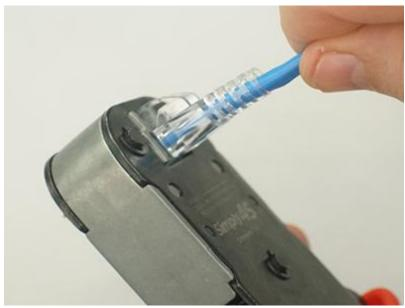
Make sure plug goes completely inside the crimping socket.
