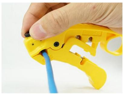
Using the Adjustable Cable Stripper, strip back the cable jacket about 1.5inches (3.8cm)
