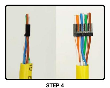
Insert the Pattern Aligned wires asshown above (B pattern shown)
