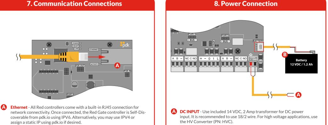
**BATTERY** - The enclosure will fit most 12 VDC 1.2 Ah batteries. The battery is connected with supplied leads and is polarity sensitive.
