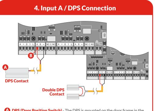
**DPS (Door Position Switch)** - The DPS is mounted on the door frame in the desired location with a 22/2 wire running from the DPS to the controller. Wire the DPS to the controller as shown above. When using two DPS sensors for double doors, you will wire them in series with only two conductors running back to the controller for connection.
