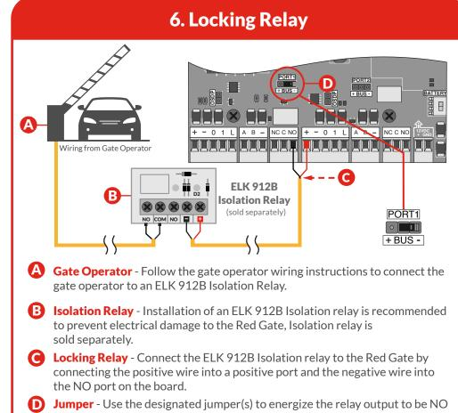
by placing the jumper on the negative (-) and center pins.
