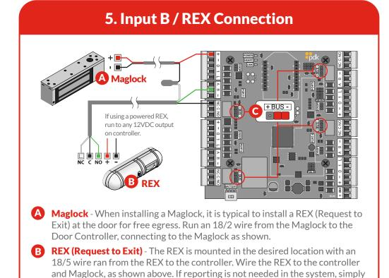
**Jumper Block(s)** - Use to designate (+) or (-) board voltage out of NO and NC.
