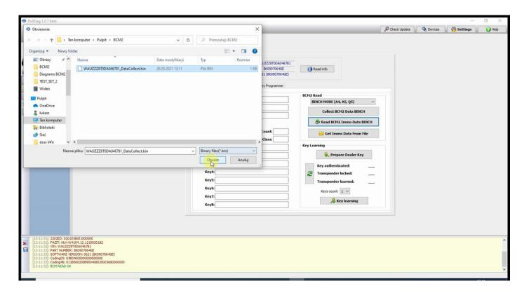
Now the software will start **BCM2 preparation** and then the **immo data extracting**. At this point, it will display **CS**, **VIN**, **MAC**, **number of saved keys and all necessary data**.
