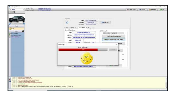
After completing this step disconnect the wires from the BCM2 and fit it back to the car. Now you can either make the **dealer key** or save the immo data for future use. **DO NOT CLOSE SOFTWARE!**
