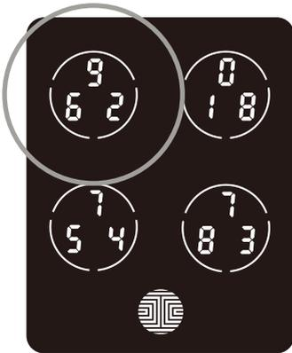
Swipe your fingers across the keypad to light up to its normal brightness. To adjust brightness, **long press the upper left button for 3 seconds.**
