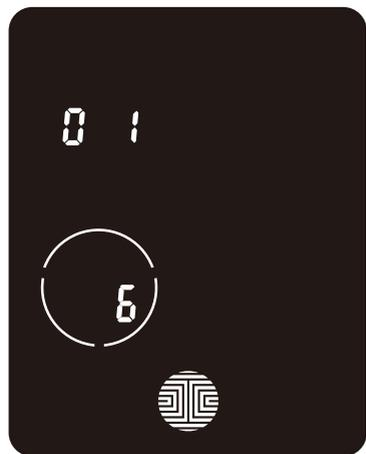
Once you're in **Fingerprint Registration Mode** you will see two numbers displayed on keypad. The top number is your **Fingerprint Registration** number, in this example to the left, **"1"**. The bottom number will always start with a **"6"**.
