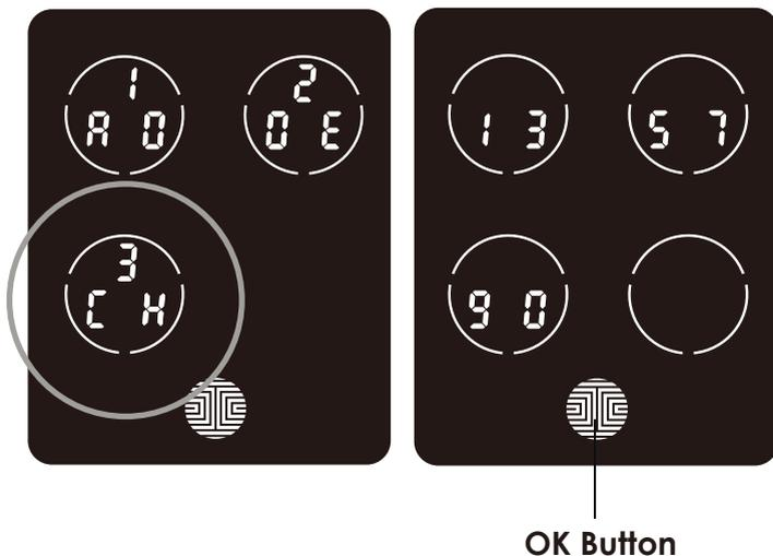
While in **Programming Mode**, select “3CH” to check registered **Access Codes**. If you are not in **Programming Mode**, please see **Section 3.2** to enter **Programming Mode**.
