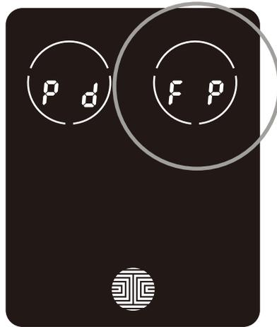
While in **Programming Mode**, select “**2DE**” to delete a **Fingerprint**. If you are not in **Programming Mode**, please see **Section 3.2** to enter **Programming Mode**.
