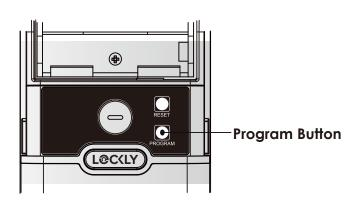
To enter **Programming Mode**, remove the battery compartment cover on the interior side of the Secure to expose the **Reset** and **Program** buttons.
