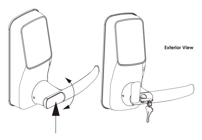
To **unlock** your lock using the **physical key (included)**, open the key cover on the handle by turning the cover to reveal the **keyhole**.
