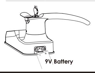
Your LOCKLY will automatically detect battery polarity. So hold your 9V battery lead in place against bottom of the LOCKLY to **temporarily** activate the screen to enter your **Access Code**. Be sure to hold the 9V battery against the contact points located at the bottom of the lock until you have successfully unlocked your door with your **Access Code**. Once unlocked, batteries should be replaced immediately.
