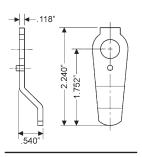
**720-3-3** inbent cam for inverted function
