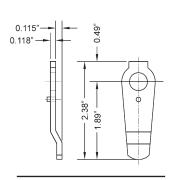
**720-3-5** inbent cam for inverted function
