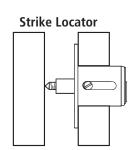
Use strike locator to correctly mark location to install strike.
