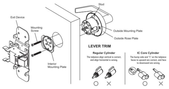
Alignment studs must enter into 5/16" (8mm) field drilled holes on outside of door. (Existing slots can be elongated with a file.)
