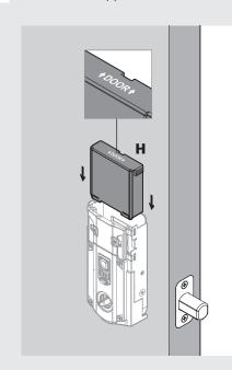
After a few seconds, the latch bolt will retract and extend on its own to learn the orientation of the door. This is called the *door handing process*, and it is crucial to lock operation.
