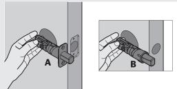
Is the D-shaped hole centered in the door hole?
