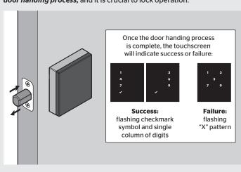
If the touchscreen indicates a failure make sure that the cables are connected, the batteries are installed correctly, and attempt this procedure again.
