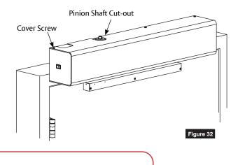
WARNING: Make sure no wiring is loose or can be caught by cover when it is snapped into place.
