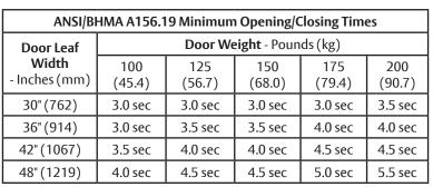
Backcheck: Adjust backcheck to have minimum opening time to backcheck or 80 degrees (whichever comes first) based on Table.
