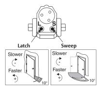
A.D.A. requires that from an open position of 70°, door will take at least 3 seconds to move to a point 3" (75mm) from latched position, measured at leading edge of door.
