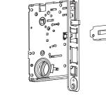
Pull latch bolt out of lock
