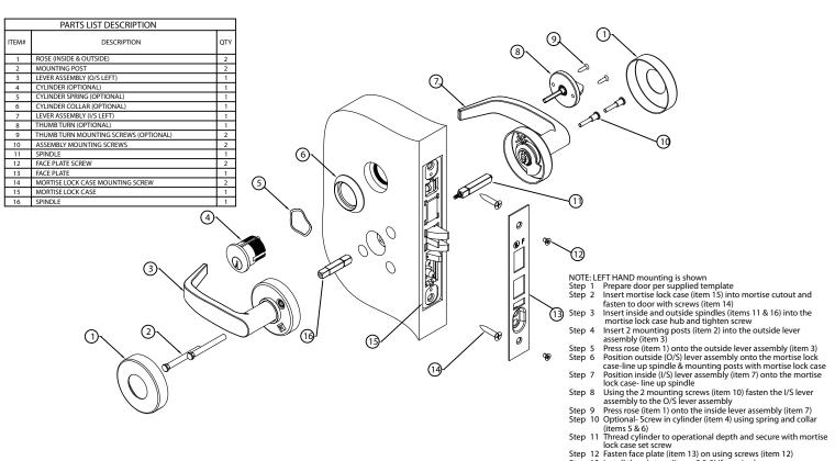
Step 12 rasterinate piate (tiefin 15) on Sing Sciews (tiefin 12) Step 13 Install thumb turn (tiens 8 & 8) if required Step 14 ALWAYS CHECK OPERATION OF LOCK SET PRIOR TO LOCKING/ SHUTTING DOOR TO CHANGE HANDING: REVERSE INSIDE & OUTSIDE LEVER ASSEMBLIES (items 3 & 7) & CHANGE MORTISE LOCK CASE HANDING
