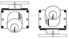
**STRIKE INSTALLATION:** Line up center mark on latch with center mark on strike for correct strike placement.
