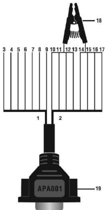
Figure 2-5 EEPROM Clamp Integrated MC9S12 Cable
