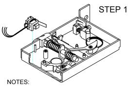
INSTALL S7800-REX INTO CASE WHERE SHOWN MAKING SURE HOLDER IS PROPERLY SEATED IN THE HOLE.
