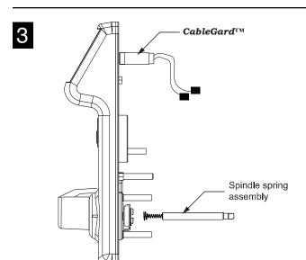
After the lever is assembled, insert spindle spring assembly into rotating hub. For alignment of spindle and hub, see below.
