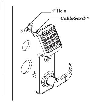
Pass the cable assembly with connectors through the 1" hole. Then place the outside trim assembly on the door.
