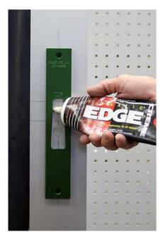
We recommend the area to be routed be lubricated with a cutting lube. We use a product called Tapmatic Edge Cream made by the LPS Company. You can find this product at industrial hardware stores or machine shop supplies. This is also a handy product to use for other drilling or tapping chores.
