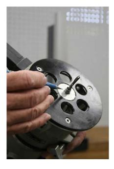
Your router needs to be equipped with a 3/8" outside diameter template guide mounted in its base. Failure to use a template guide will cause the opening being routed to be too large and will damage your HIT-40 template.
