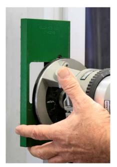
Place the router bit in the starting hole and with firm control of the router follow the HIT-40 template and feed the router slowly in a **CLOCKWISE DIRECTION**.
