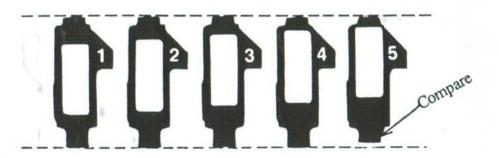
Often I have found in the first position of the door and trunk a #5 wafer substituted for a #4 wafer. This key cut position is not used in the ignition. My warning is; if Ford substitutes a #5 wafer for a #4 wafer in any other door or trunk position when you have fully progressed the ignition key it will not work the ignition! At this point suspect all #5 cuts in positions #5 thru 9. One or more of them may be a true #4 code cut.
