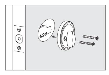
Mount thumb turn assembly on door, aligning onto latch crank, tighten screw firmly to secure assemblies to door.
