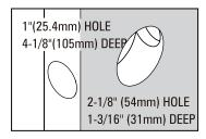
Drill 1" (25.4mm) hole 4-1/8" (105mm) deep in center of door edge. Drill from room side or inside of door 2-1/8" (54mm) hole 1-3/16" (31mm) deep on door face.
