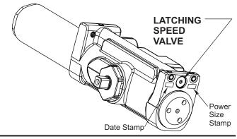
**Backcheck Location Valve** (3/32 Allen Wrench Provided) Valve is closed, as shipped, from factory. To increase the degree of door opening where backcheck takes effect, turn valve counter-clockwise.
