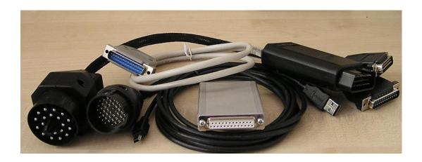
**Powering up the device.** CarProg can be used with external power supply (+7 - +12V stabilized), only with USB connection or with diagnostic cable ( for ex. OBDII)
