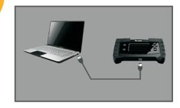
Connect the PC and the IFIX main unit with the USB cable before software update
