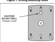
Figure 1: Drilling Mounting Holes
