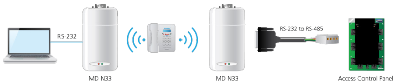
Figure 24: Remote Site Modem Configuration
