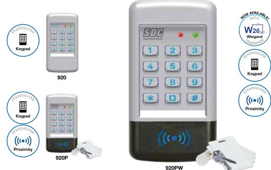
The SDC EntryCheck<sup>™</sup> 920 Series indoor/outdoor digital keypads are designed to control access of a single entry point with up to 500 users. Each user is assigned a personal identification number (PIN). Keypad entry of a valid one to six digit code activates one or both of the output relays which releases an electric door lock. Featuring heavy cast vandal resistant housing and cast metal blue backlit keys.
