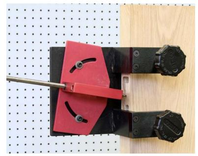
A 3/8" rod (supplied) inserted into the hardened drill guide to show where drill bit will make contact to door.
