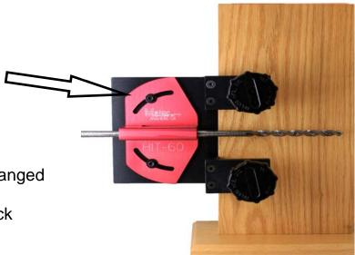
The drilling angle can be changed by using a 3/16" hex key to loosen the drilling guide block and tightening after adjusting.
