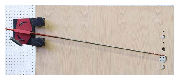
The full length drill bit inserted in the drill guide. By having the 3/8" rod and drill bit inserted at the same time, you can see where the drill bit will make contact to the door and where the hole will end up.
