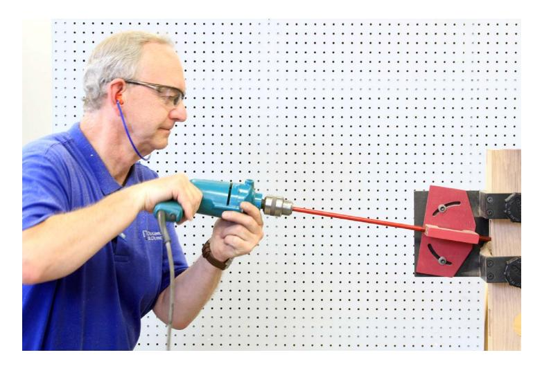
Once you have drilled about a quarter of the way through the door, run the drill bit to the bottom of the hole and pull completely out with the drill still running. Do this step several times through the rest of the drilling procedure. This will keep the chip buildup clear through the rest of the drilling.
