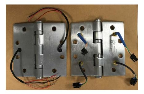
Standard electrified hinge prep used by most hinge manufacturers. These hinges require just a round hole (typically 5/8" diameter, 1-1/2" deep) for the wire service connection. The wire service connection is just a pocket where the wires are connected.
