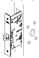
2. Insert lock and fasten with two screws.
