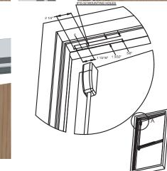
Option just to use the dimensions below to mark the mechanism hole and the mounting screw positions. Use a #10-32 tap for the mounting screw thread.
