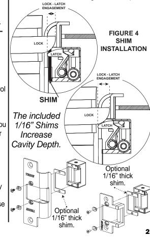
The 323478F-LC kit's 234 Faceplate is horizontally adjustable. In this illustration, the mechanism is mounted on a normal position.
