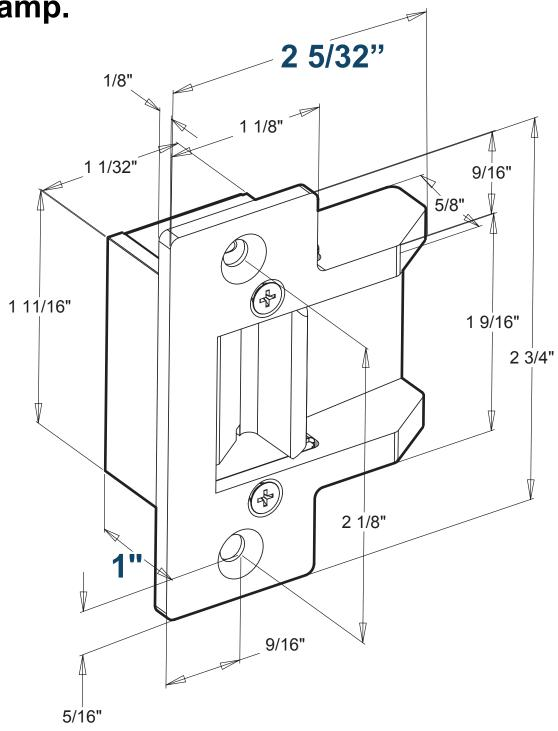
NOTE: USE 2 INCH LONG (OR LONGER) WOOD SCREWS FOR MOUNTING IN WOOD FRAMES
