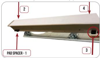
**9.** Re-install the **Push Pad Assembly** into the exit device housing, keeping an eye on the push pad spacer & rubber bumpers.
