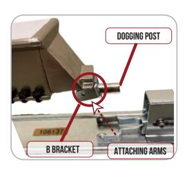
6. Once Attaching Arms are lined up **insert (C) PIN** to connect to (B) bracket.
