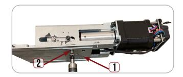
5. Slide the (B) Connecting Bracket over the Dogging post at the end of the push pad. Next, move Attaching Arms on motor kit up to line up with holes on B Bracket.
