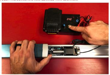
17. FIRE OFF THE DEVICE A FEW TIMES TO ENSURE THE LOCATION IS CORRECT. AFTER INSTALLING THE DEVICE ON THE DOOR, RECHECK TO VERIFY THE PUSHPAD IS RETRACTING TO THE DESIRED LOCATION. IF NOT, REPEAT STEPS 15-16.
