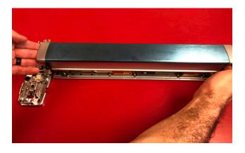
5. IF YOUR DEVICE HAS DOGGING, FLIP BASERAIL OVER & REMOVE (2) SCREWS SECURING DOGGING ASSEMBLY TO RAIL. IF YOU HAVE AN OLDER DEVICE WITH RIVETS, YOU WILL NEED TO DRILL THEM OUT OR USE A PIN PUNCH TO KNOCK THEM OUT.
