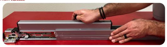
12 FLIP OVER RE-INSTALL (4) SCREWS TO SECURE BASERAIL TO HOUSING.
