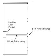
**STEP 2**: Run the wires from the ETH hinge through the 3/8" raceway starting at the ETH hinge & exiting into the mortise pocket.
