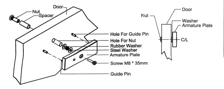
Fix the armature plate not too tightly, and make the rubber washer more flexible, in order to make the armature plate automatically adjust its proper position with the magnet.
