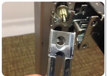
C. Reinstall Axle screw and tighten.
