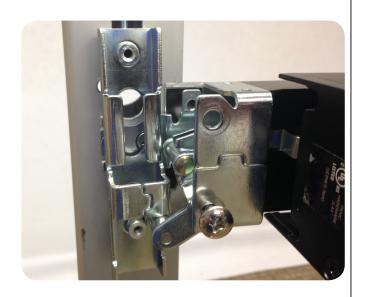
D. Install Pinion support bracket and tighten retainer screw.
