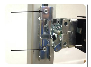
C. Re-install Axle screw and tighten.
