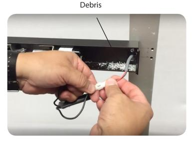
Note: Depending on where your power transfer is; next you would fish the other side of the power lead we connected to the MM4 and hook up to your incoming power. If you have a portable tester this would be a good time to test fire the motor.
