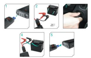
Check the level of battery of jump starter. To start the vehicle, it is necessary to have a capacity of at least 3-4 LEDs in the battery indicator (3). New jump starter must be charged before usage
