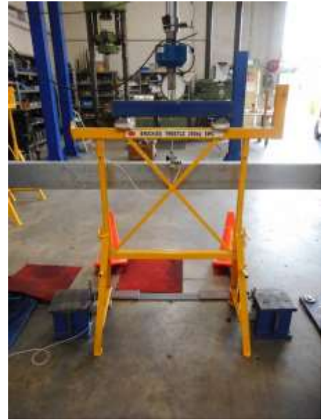
FIG. 3 STRENGTH TEST SET-UP
